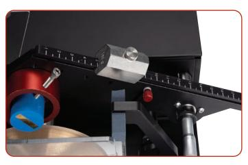
Sliding weights with graduated arm indicators provide variable load.
