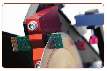
Fixtures are adjustable to optimize the cutting angle.
