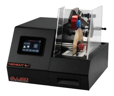
The **TechCut 4x**<sup>™</sup> is a precision low speed saw designed to cut small or delicate samples that cannot tolerate increased heat from friction caused by high speed sectioning.
